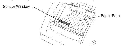
**2.** Remove dust from the Media Sensor with a brush or equivalent.
